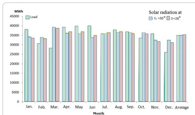
Figure 4: Monthly load distribution and the solar radiation on tilted surface, 30° and 26° for Brack El-Shati-Libya.
